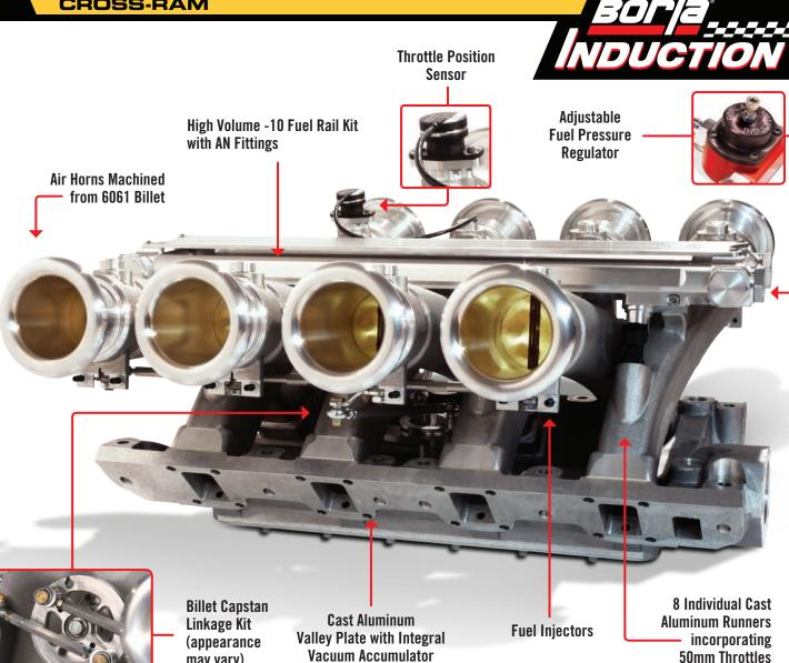
BORLA® Induction presents a real cross-ram manifold for the Ford 351 Windsor small block engines fitted with 8 long runners for stump-pulling torque. Our valley plate incorporates a vacuum accumulator and its extended port wall construction enables machining for several different port configurations from OEM to 225's. Boasting looks to die for and ground-shaking power, our Ford Cross-Ram kit was voted one of SEMA's Best New Products for 2009.
